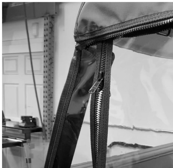
Step 6: Align LH quarter panel with LH side panel to ensure zipper engagement, close zipper. Firmly install panels to rails and closeout. Repeat on right side
