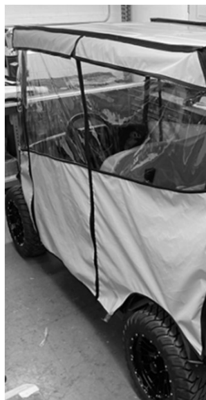
Step 6: Loosely install LH side panel to LH rails. Repeat on right side
