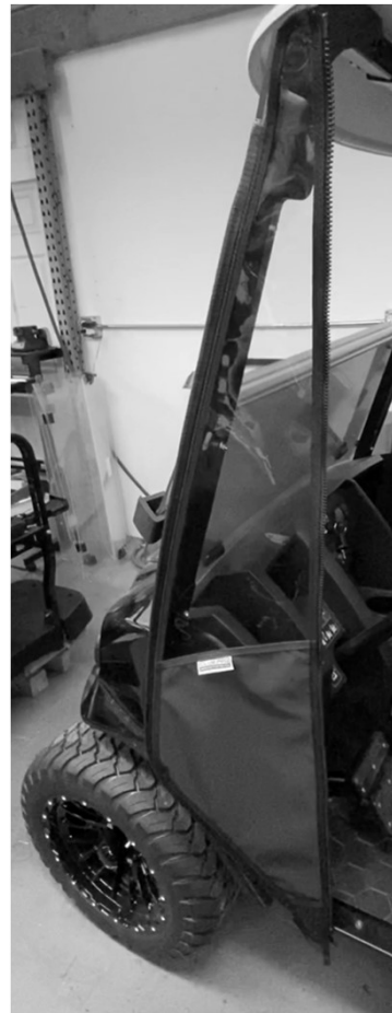
Step 5: Loosely install LH front side quarter panel to closeout. Repeat on right side
