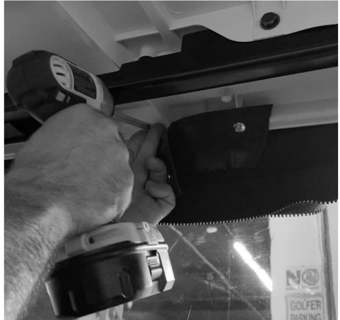
Step 8: Install self tapping snaps in line with gutter flap. Close snaps to secure gutter to canopy
