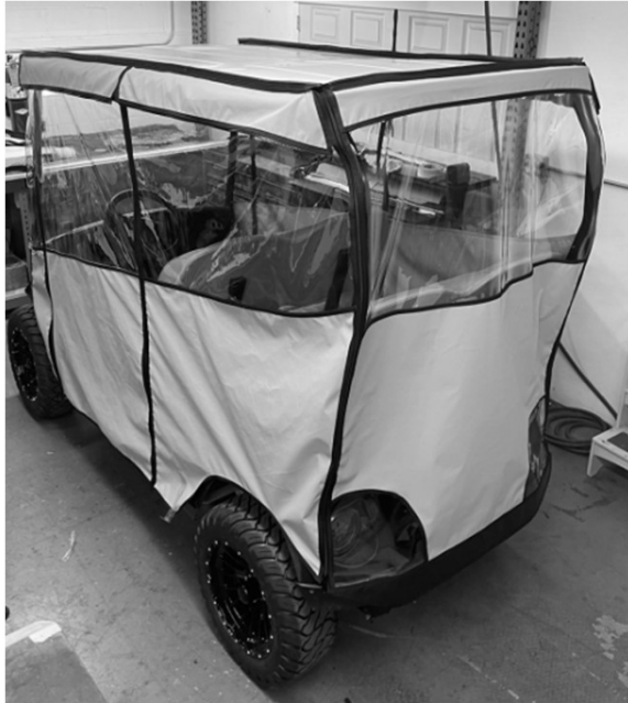
Step 7: Install rear panel to cross car rail, engage zippers, close zippers
