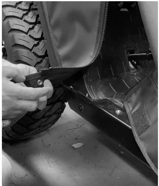
Step 9: Clean rocker panel, apply 3M primer to rocker panel, assemble male snap to fabric as shown, remove backing paper, press snap against rocker panel and apply pressure for 30 seconds. Leave snapped for 1 hour, repeat on right side.
