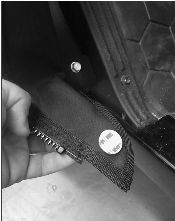
Step 9: Clean rocker panel, apply 3M primer to rocker panel, assemble male snap to fabric as shown, remove backing paper, press snap against rocker panel and apply pressure for 30 seconds. Leave snapped for 1 hour, repeat on right side.
