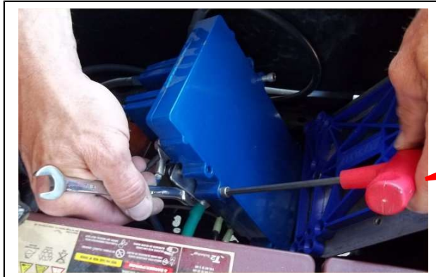
Install mounting bolt from bottom through the controller and TOW/RUN bracket
